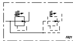
FR21 = Manifold regulator without relieving and without pressure gauge
